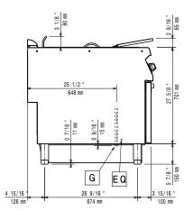
EQ = Equipotential screwG = Gas connection
